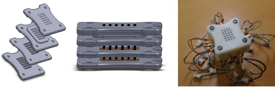
Fig. 1. Implemented 6 by 4 pin array vibrotactile stimulator that has 2.9mm pitch. The stimulator consists of four layers (left) and the motors are placed over two layers (middle) for the minimum pitch. Frame is built using acrylic resin material and total dimension is 40mm x 40mm x 17mm (right).
